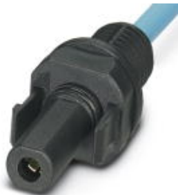
Photovoltaic connector, nominal current: 40 A, nom. voltage: 1500 V, connection method: Crimp, color: black. Can only be released using a tool
