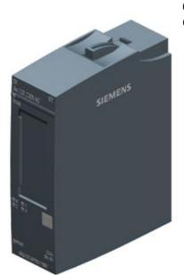
SIPLUS ET 200SP, Digital input module, DI 4x 120..230V AC ST, type 3 (IEC 61131) -40...+70°C with conformal coating based on 6ES7131-6FD01-0BB1 . Packing unit: 1 piece, fits to BU-type B1, Colour Code CC41, module diagnostics
